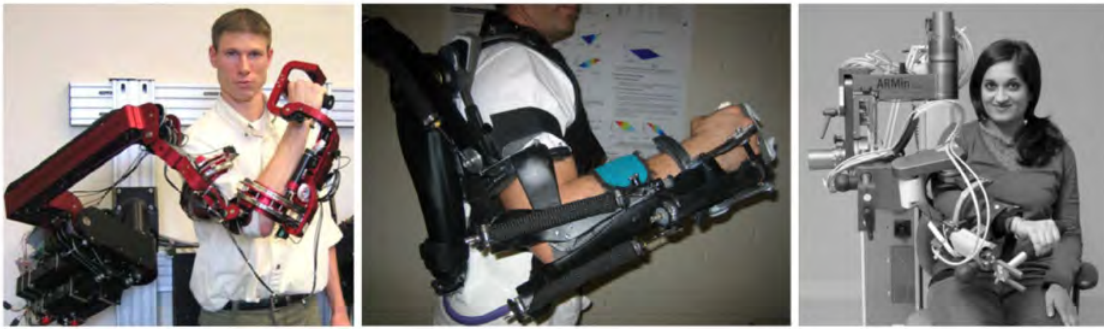
Figure 2.6: Examples of exoskeletons with various DOF, the first one is CADEN-7 [32], second RUPERT IV [33] and the last ARMin III [34]
