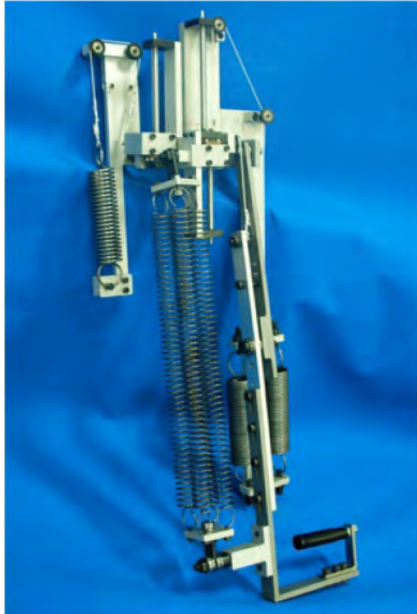
Figure 2.1: Example of passive exoskeleton based on springs [20].
