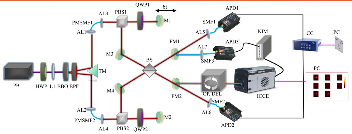
Fig. 1: Experimental setup to observe HOMI using an ICCD working in coincidence.
