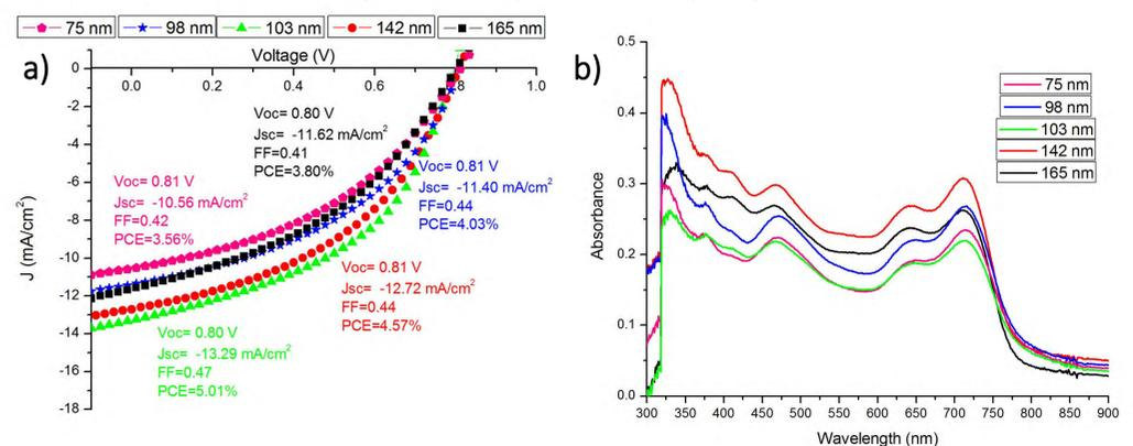
Fig. 5: (a) J-V curves of solar cells with different active layer thicknesses, (b) Active layers absorbance
