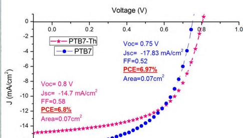
Fig. 3: Best efficiencies obtained with PTB7 and PTB7-Th
