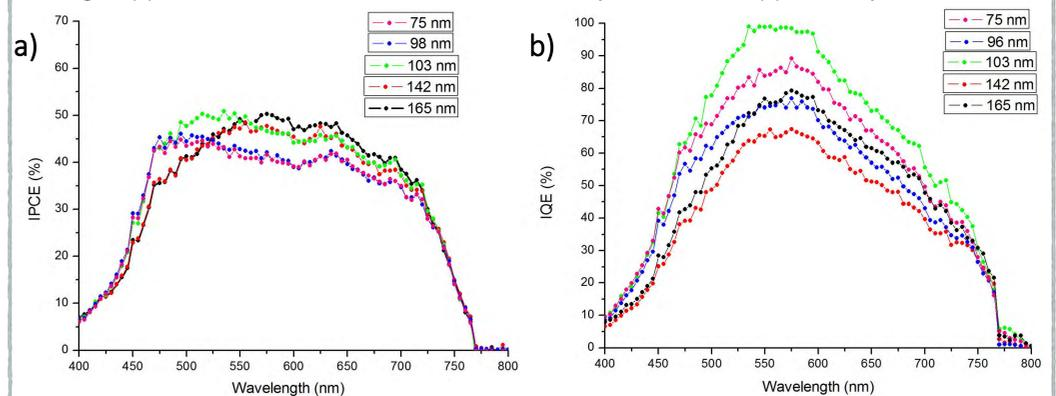
Fig. 6: (a) IPCE and (b) IQE curves of solar cells with different active layer thicknesses
