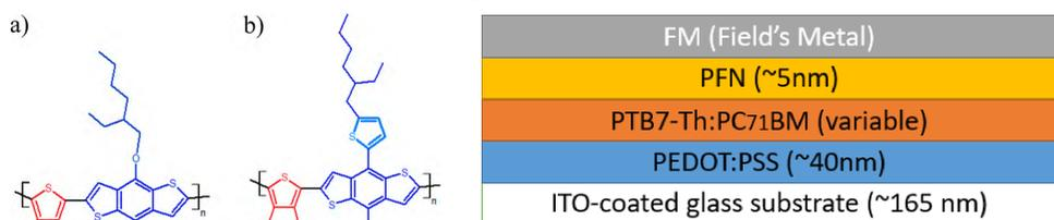
Fig. 2: (Left) Chemical structure of (a) PTB7 and (b) PTB7-Th, (Right) Scheme of OPV's
