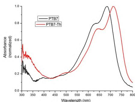
Fig. 4: Absorption spectra of PTB7 and PTB7-Th films
