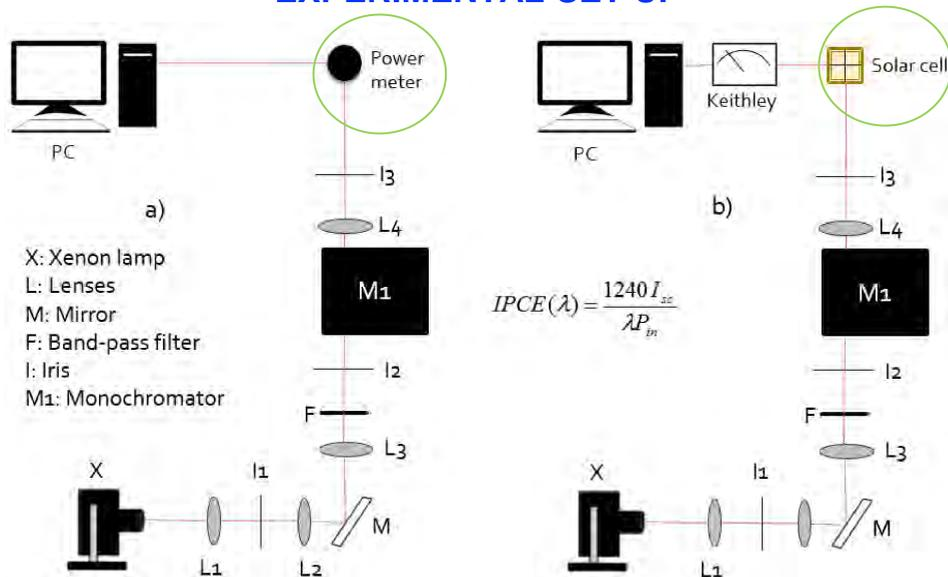
Fig. 1: IPCE scheme: a) Power measurements, b) solar cell current measurements
