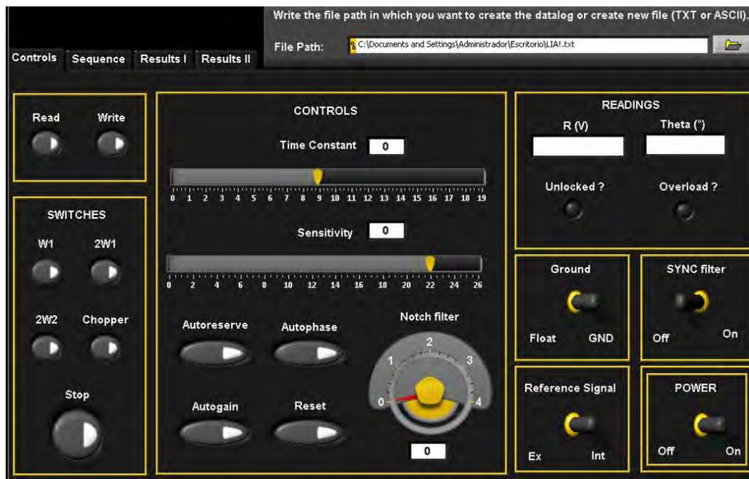
Figure 3.18 – Control panel for manual operation of system
