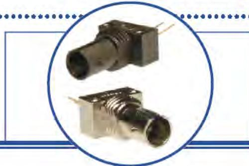
The OPF692 and OPF693 fiber optic transmitters are high performance devices packaged for data communication links. These transmitters are an 850nm GaAlAs LED and are specifically designed to efficiently launch optical power into fibers ranging in size from 50/125µm up to 200/300µm diameter fiber. Multiple power ranges with upper and lower limits are offered which allows the designer to select a device best suited for the application.
