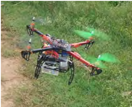
Figure 1.13: Quad-rotor for the implementation of an imaging system used in [3].
