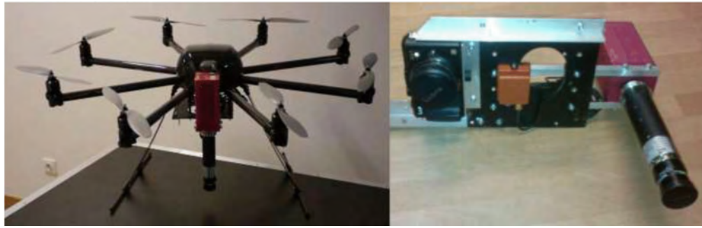
Figure 1.6: Hyperspectral imaging system implemented on a octa-rotor.
