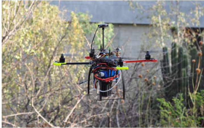
Figure 1: The unmanned aerial vehicle used in this work. This drone is equipped with the proposed multispectral imagery system.
