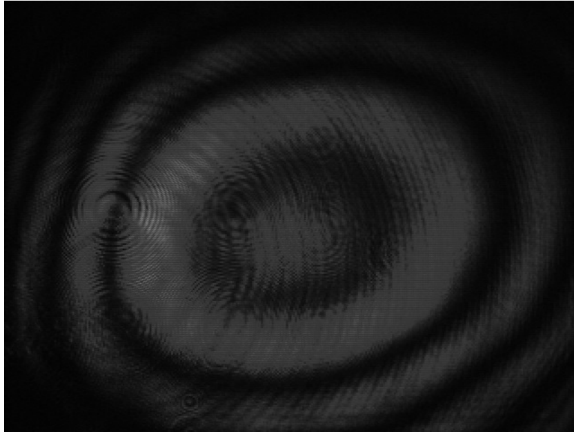
Figure 5.1.1. Fringe pattern I_0 produced by the implemented interferometer displaying the gray level zero on the SLM.
