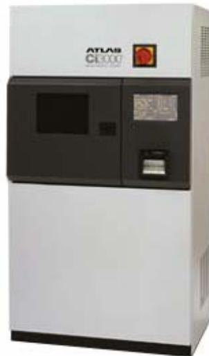
Fig. 3.5 Weather-o-meter modelo Ci3000 de Atlas Electric
