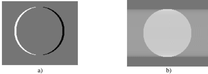
Figure 4.3 a) Constat wave-front lateral shearing along x -direction with k_x=2 CCD pixels and b) Wave-front recovered using the simple inverse transfer function.
