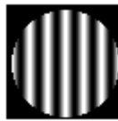
Figure 1.4 Interferogram produced by defocusing
