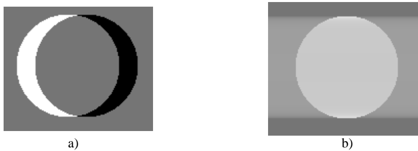
Figure 4.4 a) Constat wave-front lateral shearing along x -direction with k_x=9 CCD pixels and b) Wave-front recovered using the simple inverse transfer function.
