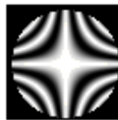
Figure 1.7 Interferogram produced by Coma aberration, Sagittal Shear
