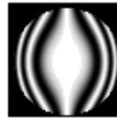
Figure 1.5 Interferogram produced by Spherical aberration
