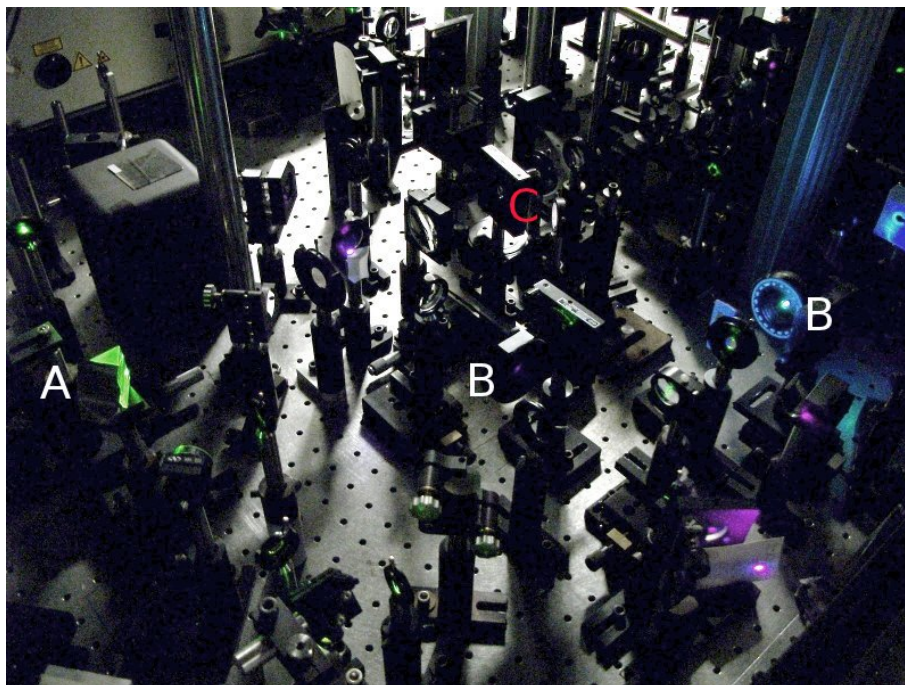
Figure 3.4: The NOPA at the Femtosecond Spectroscopy Lab. One prism (A), two crystals (B), and the sapphire window (C) can be seen.
