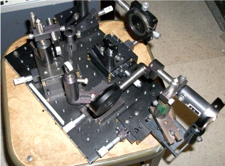
Figure 3.5: Second XP2SHG breadboard. Substrate sample in holder and BBO crystal folded away at middle.
