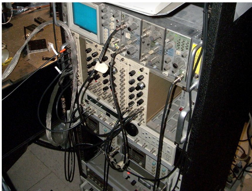
Figure 3.9: Electronics for detection equipment. From bottom device with red light: power supply for PMTs, HP Voltimeter, Stanford Research SR400, Ortec 401A, and Tektronix 7903 oscilloscope. In Ortec rack from left to right: SR240 Fast Preamp, 2 × SR250 Gated Integrator, SR245 Computer Interface, and SR250.
