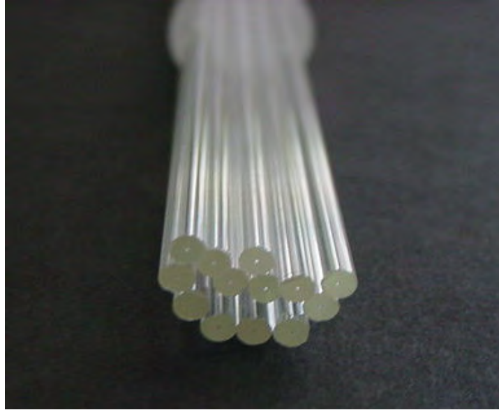
Figure 2.7 Silica thin capillaries are placed into a preform
