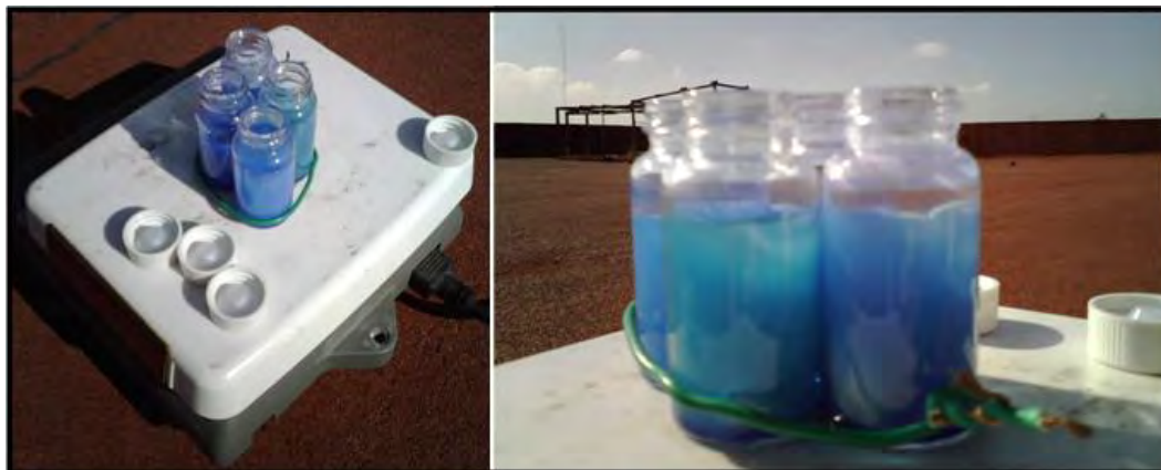
Fig. 40 Set up for photodegradation of MB solution by Ba(Zr) 1-x Bi x O 3 ( x= 0, 0.1, 1 and 10 ) photocatalyst activated by natural sunlight irradiation.
