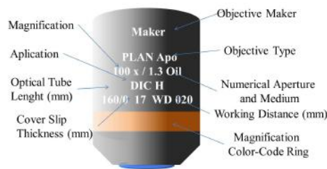
Figure 1.3. Typical microscope objective nomenclature.
