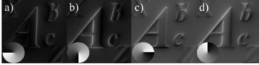
Figure 2.14. Intensity distribution I^{(n)}(x_i, y_i) for a weak phase object. a) I^{(1)}(x_i, y_i) , \alpha_1 = 0 , b) I^{(2)}(x_i, y_i) , \alpha_2 = \pi/2 , c) I^{(3)}(x_i, y_i) , \alpha_3 = \pi , d) I^{(4)}(x_i, y_i) , \alpha_4 = 3\pi/2 .
