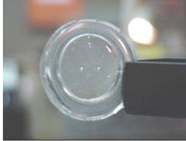
Fig. 1. A fabricated flexible lens
