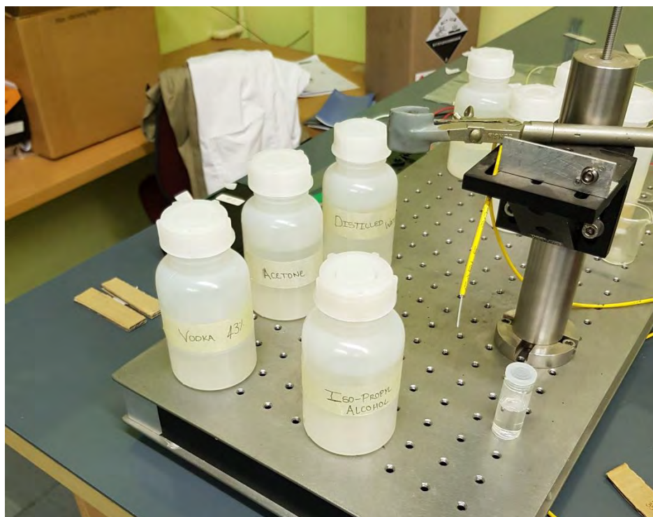
Figure 67: The dipping platform with the different chemicals that were measured (glycerin is in the small container)
