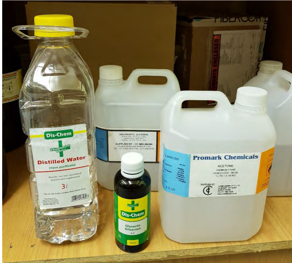
Figure 61: Some of the chemicals used for refractive index measurement, e.g. distilled water, iso-propyl alcohol, glycerin and acetone
