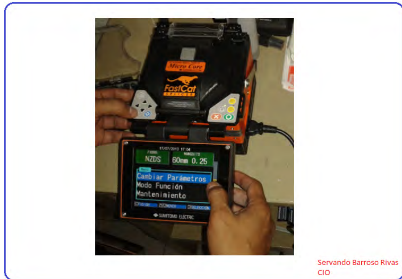
FIG. 3.14 EMPALMADORA FASTCAST SPLICER.
