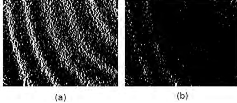
Figure 4.4: Phase difference with respect to x (partial approximated derivative). The dynamic range of the difference is quantized to the gray levels 1, 102, 153, 203 and 255, for a better appreciation of the detuning error. (a) shows the phase difference corresponding to the AIA and (b) shows the difference corresponding to RAPS method.
