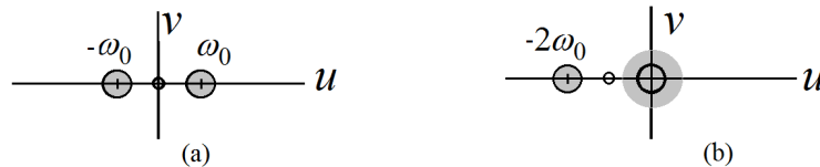
Fig. 2. In panel (a) we show the Fourier spectrum of the real-valued phase-modulated fringe pattern. In panel (b) we show the frequency-shifted spectrum and the low-pass filtering as a gray disk at the spectral origin.
