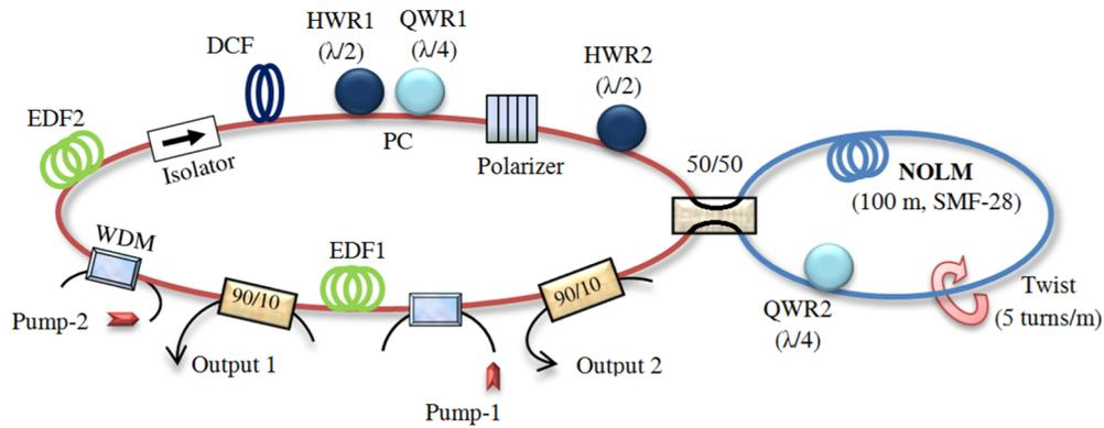
Fig. 1. Scheme of the figure-eight fiber laser.
