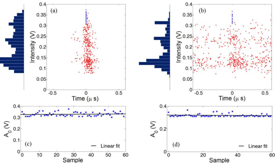
Fig. 4. Statistical analysis of the energies of the sub-pulses (a) when the drifting sub-pulses decay and finally disappear and (b) when the sub-pulses drift throughout the cavity; (c) and (d) Energy of main pulse extracted from data in (a) and (b), respectively.
