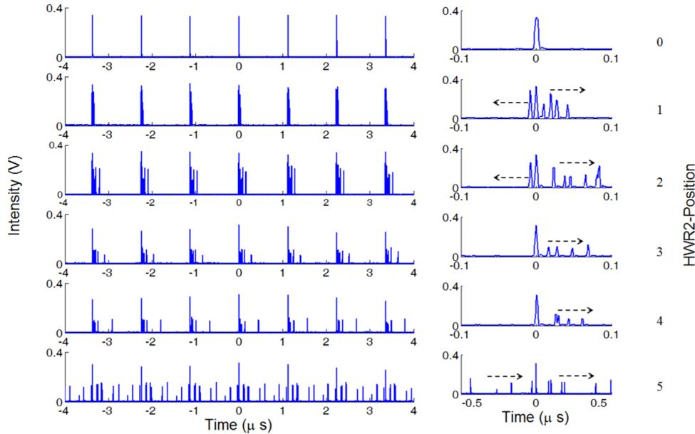
Fig. 3. Evolution of the NLP dynamics observed with a 2-GHz photodetector and 200-MHz oscilloscope in single-shot mode, as the position of HWR2 is varied: the left figures display  $\sim 7$  cavity periods, and the right figures present a close-up on the central portion of each trace. The arrows indicate the direction of propagation of the sub-pulses released by the central waveform. See also [Visualization 1](#) and [Visualization 2](#).
