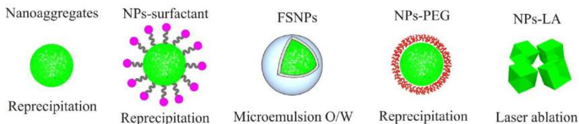
Fig. 3.2 Architectures of organic fluorescent nanostructures and their fabrication methods. NPs-PEG could have different functions in the block sections or simply to self-assemble into uniform structures and silica shell in FSNPs acted as protecting agents of matrix or scaffold, which thus offers better functionalization and biocompatibility.
