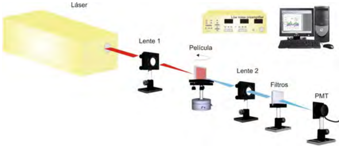
Figura 6.21. Arreglo experimental de THG Maker-Fringes.
