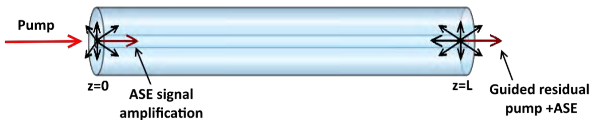
Figure 6.6. Processes of pump absorption and ASE generation along a doped optical fiber.
