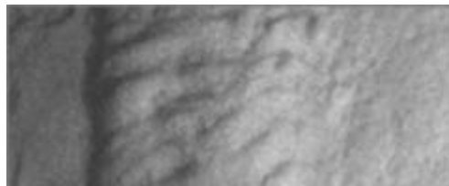
Figure 3.7 Surface with abrupt relief. Illumination array was performed in order to avoid shadows introduced from the central relief.
