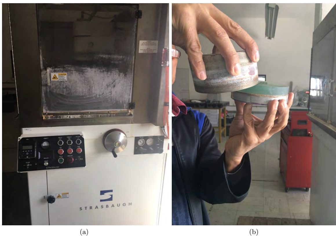
Figure 7.5: Generating machine.a) Machine,b) How mechanical tool makes contact with glass to generate a spherical lens.
