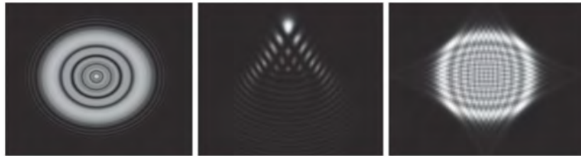
Figure 2.8: Diffraction pattern in presence of spherical aberration, coma and astigmatism aberrations
