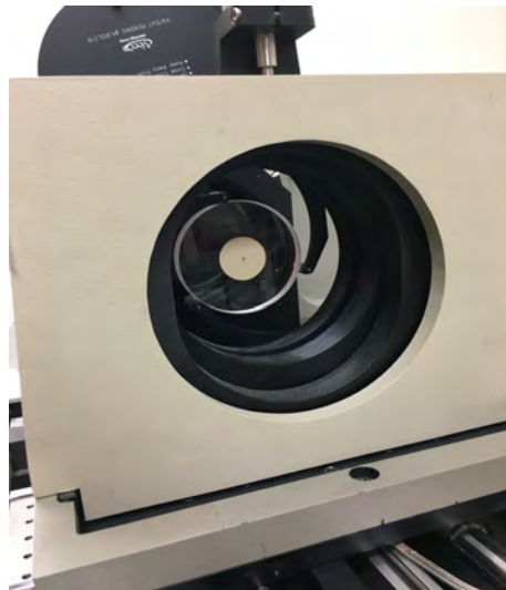
Figure 4.11: Circles acting as amplitude pupils placed on the lens.
