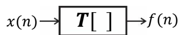
Fig. 2.3.-Representation of a transformation that maps an input sequence x(n) into an output sequence f(n) .
