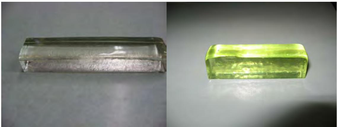
Figure 1.3 Bulk samples of a) phosphate and b) tellurite glass after annealing.
