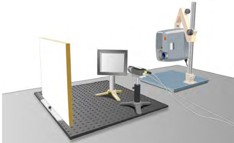
Figure 4.4: Experimental setup that consists of a reference plane, a CCD camera, a projector and a beam splitter 70:30.
