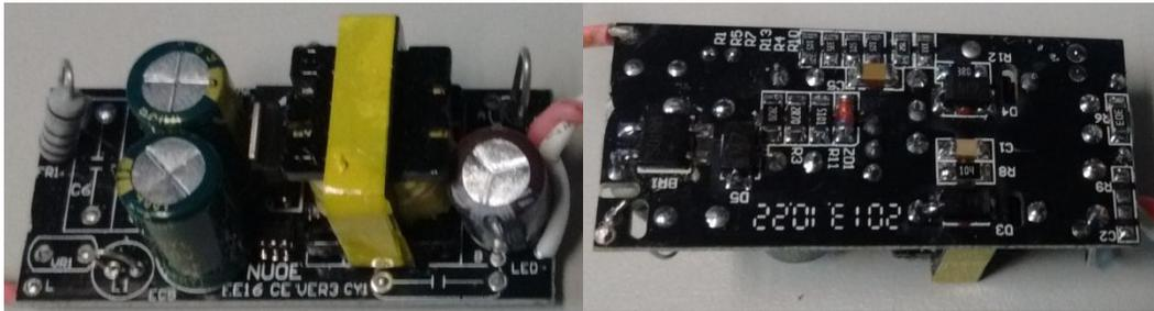
**Figura 3.42.** Driver lámpara LED Smartlight 7 W.
