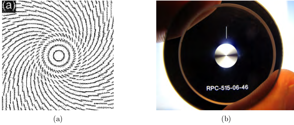
Figure 2.4: a) Geometrical disposition of the nano gratings in the s-wave converter. Taken from Beresna and Kazansky (2014). b) Photograph of the S-waveplate between crossed polarizers. Taken from the web-page of Altechna.
