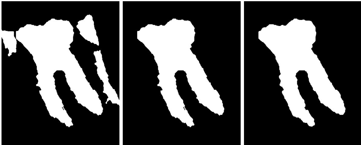
(e) Morphological closing with structuring element of type line , length = 10 px, angle = 120^\circ .
