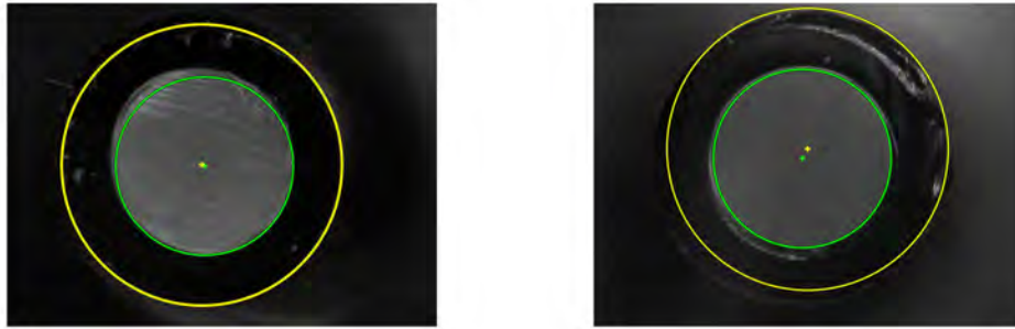
(a) Concentricity displacement of \approx 15 \mu\text{m} . (b) Concentricity displacement of \approx 55 \mu\text{m} .
