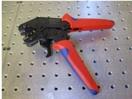
Figure 28: Specialized stripping and cutting tool for MOST POF.
