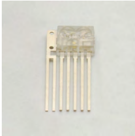
Figure 23: MOST 150 Mbps transceiver by Hamamatsu. Adapted from Ref. [B16].
