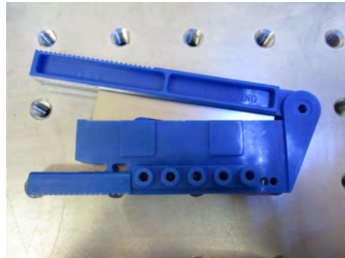
(b) Gullotine functioned razor blade cleaver.
