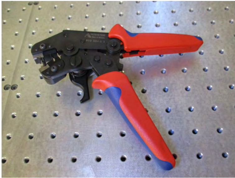
Figure 52: Specialized stripping and cutting tool for MOST POF.
