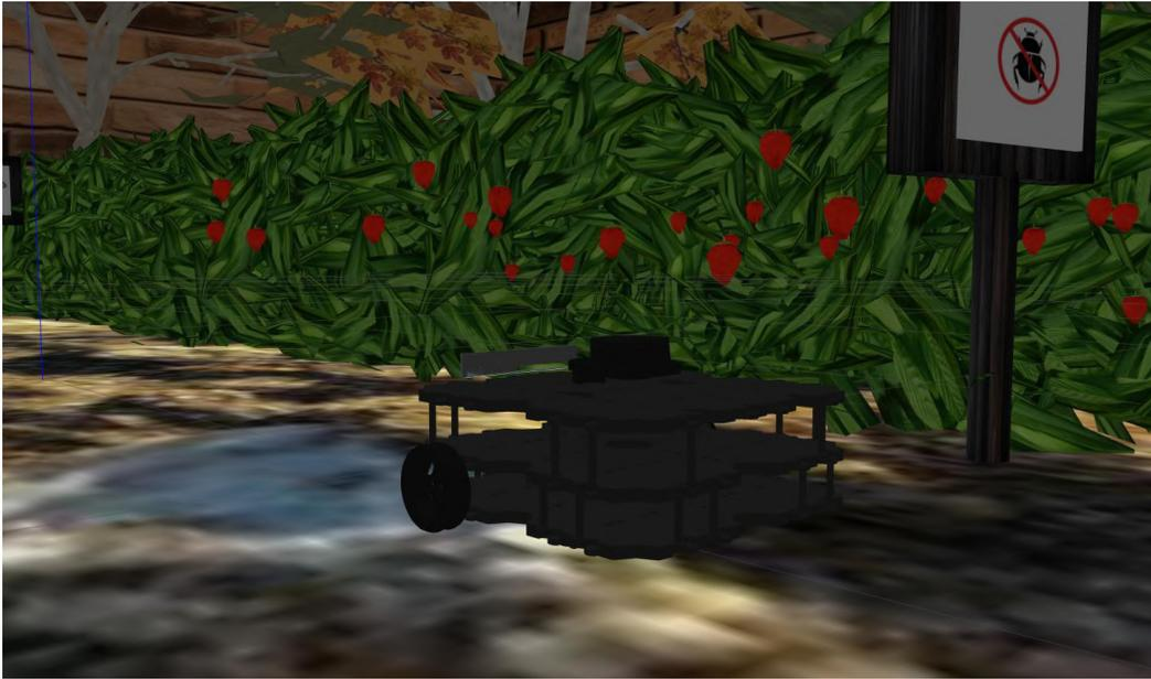
**Figure 4.1:** The TurtleBot navigates between rows of strawberries, scanning the environment. The code developed for this project is available on GitHub: [github.com/erandivg/strawberry\\_field\\_ws](https://github.com/erandivg/strawberry_field_ws)
