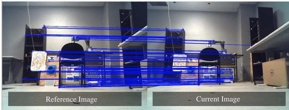
**Figure 4.9:** Point correspondence between the reference image and the current image. The detected key points in both images are used to compute the homography and determine the robot’s position.
