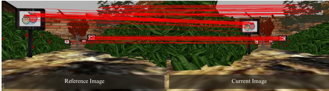
**Figure 3.4:** The image shows the result of key point matching between two views of a scene, using feature detection and description. The red lines indicate the correspondences between the detected points in both images.
