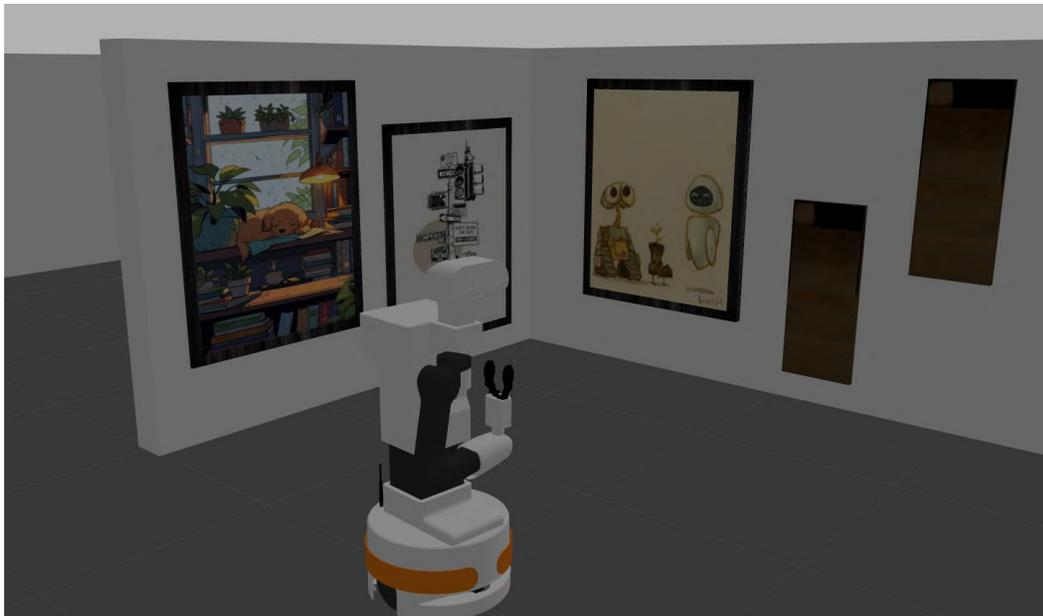
**Figure 4.6:** Simulated image of the TIAGo robot in Gazebo, showing its mobile structure with a wheeled base, a robotic arm and an integrated camera. The simulation includes a virtual environment with realistic lighting and shadows.
