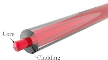
*Figure 1.1: Scheme of an optical waveguide.*
