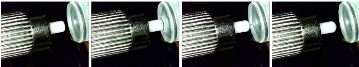
Figure 8. Real pictures of the polymer transferring process of a ferrule connector tip.
