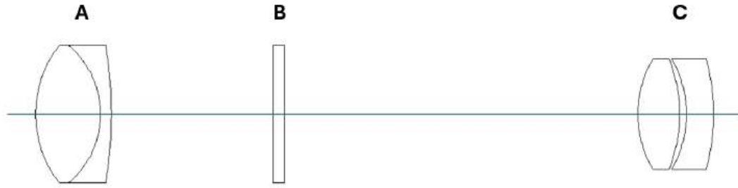
Figure 3.5 – Diagram representing the optical system simulated in Oslo. A and C represent the doublet lenses, while B is the polarizing element incorporated into the system. The wave retarder could not be included due to software restrictions.
