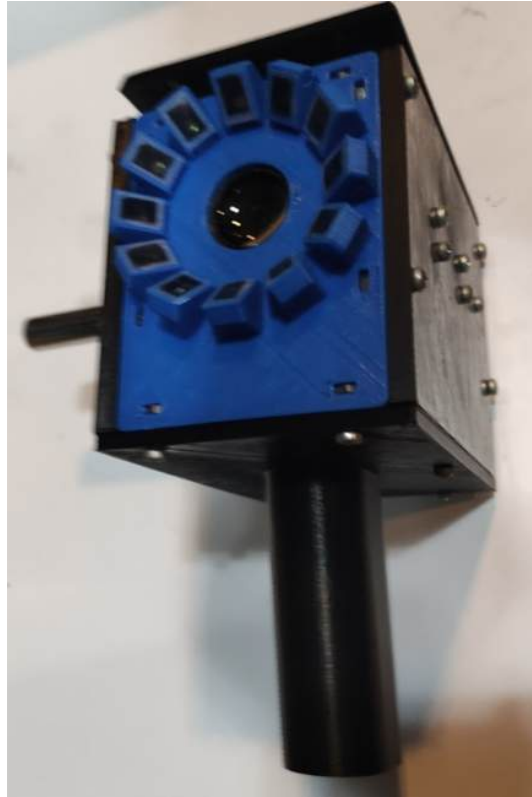
Figure 2.3 – Multispectral polarimetric dermatoscope using two rotating polarizing elements.
