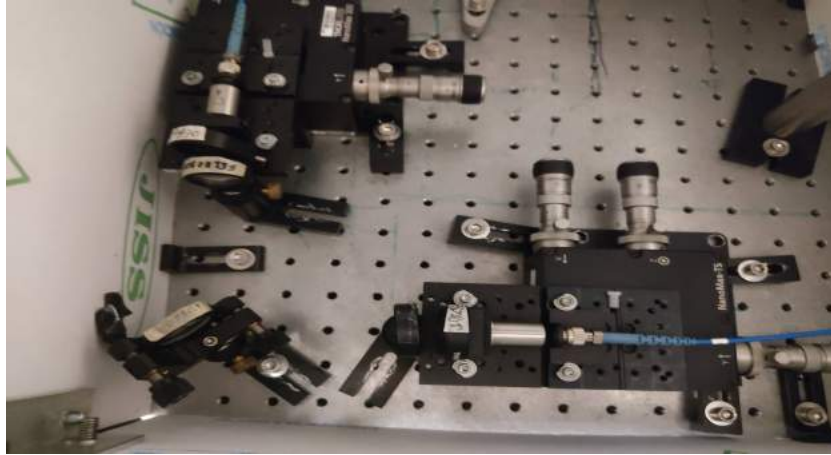
Figure 4.8: The dichroic mirror divides the Signal and Idler and both are filtered to eliminate any possible pump remaining.
