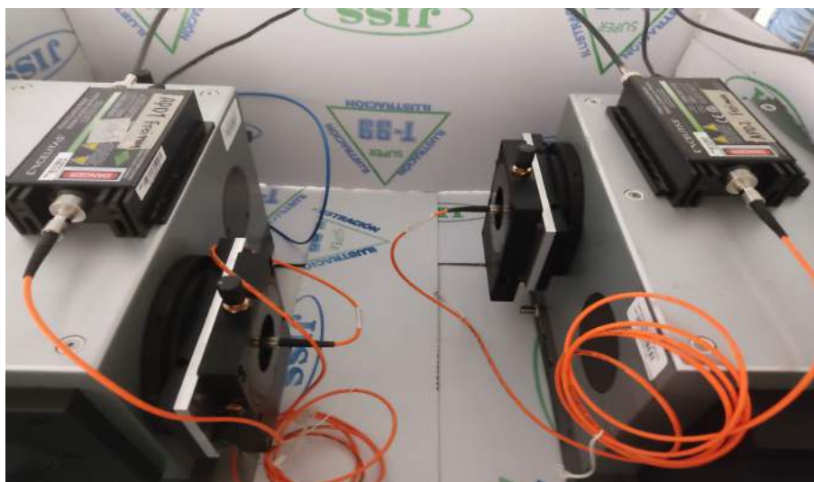
Figure 4.14: Monochromators with APDs connected, the cardboard box around was needed because there was a big amount of the laser light entering the APDs.
