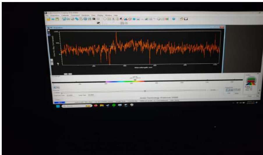
Figure 4.18: Spectra of the signal with a width of 50 ns, the width of the pulse determine the time window in which the gain is active.
