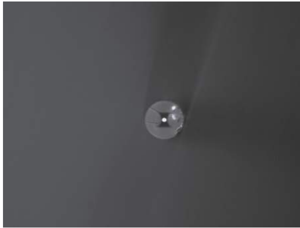
Figure 4.4: Bow-tie structure of the HB800G fiber, it was illuminated with a white light on the other face.
