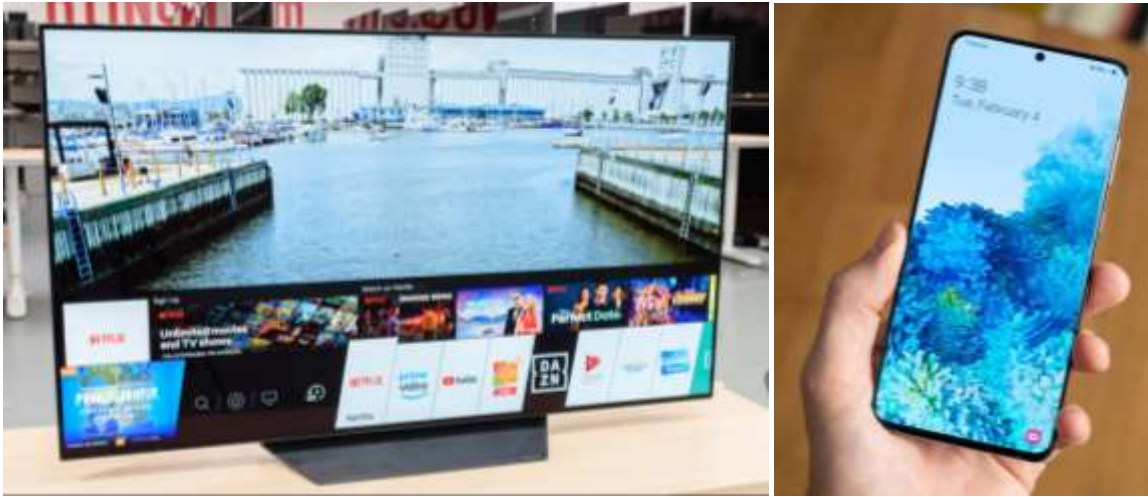
Fig. 2. LG OLED TV (B9 model 2020) with a maximum luminance of 767 \text{ cd/m}^2 and the Samsung galaxy s20 ultra with a maximum luminance of 1342 \text{ cd/m}^2 .
