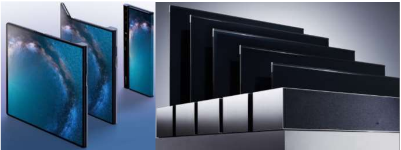
Fig. 4. Foldable OLED device Huawei Mate X and rollable OLED LG smart TV 8K.
