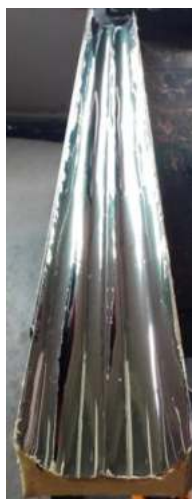
Figure 20.- Final result of the CPC Collector built with the 3D mold
