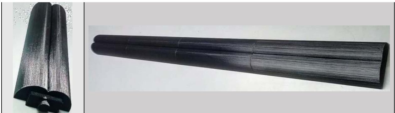
Figure 17.- 3D-Mold male piece (left) and assembled pieces forming the CPC 3D-Mold.
