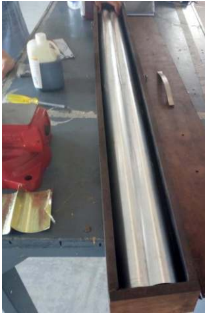
Figure 18.- 3D-Mold and aluminum sheet inside the container developed.
