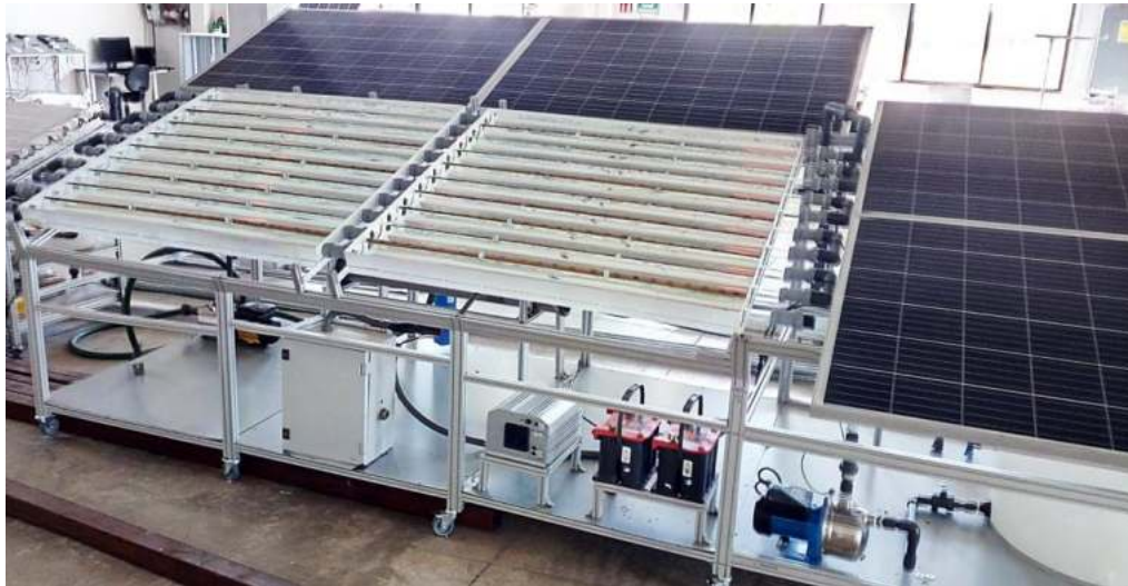
Figure 37.- CPC collectors mounted on the top of the photoreactor structure
