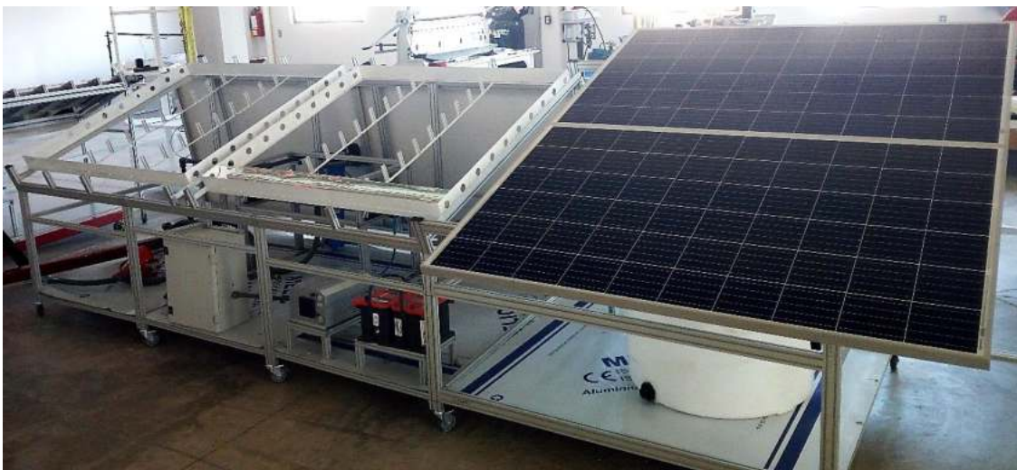
Figure 36.- Structure frames on the top of the structure (left side) utilized to mount the collectors
