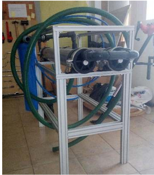
Figure 14.- Supported RO membranes on the aluminum profile structure
