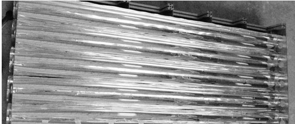
Figure 21.- Conventionally manufactured CPCs assembled in a special structure to maintain the collector shape.
