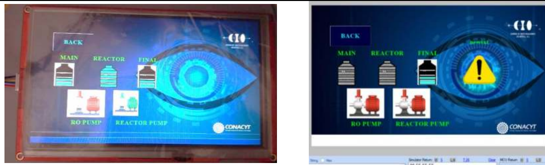
Figure 42.- Evaluating the Nextion display status in real-time (left) and virtually simulated (right).
