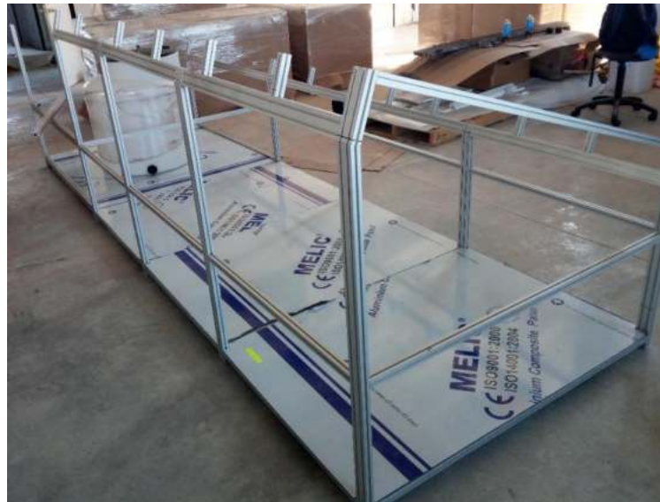
Figure 32.- Structure base for the solar water potabilizer
