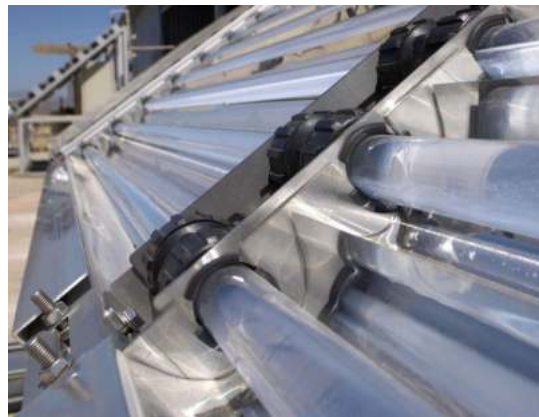
Figure 8.- CPC collectors placed in a tubular solar reactor [29]
