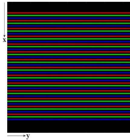
Figure 5.2. Grating of structured light with color multi-lines to project.
