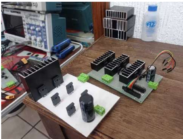
(a) Controlled three-phase rectifiers designed for different tests.
