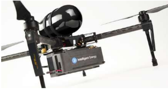
(a) Quadrotor using a fuel cell system, as a substitute for batteries, is integrated by, fuel cell, the balance of Plant (BoP), hybrid battery, hydrogen Storage [27].
