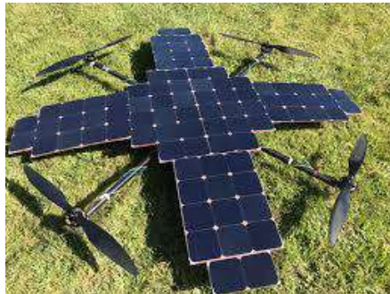
(c) Solar-powered Sentra quadrotor, these quadrotors still have limitations, because the cells must supply the power needed for the four engines at takeoff [20]
