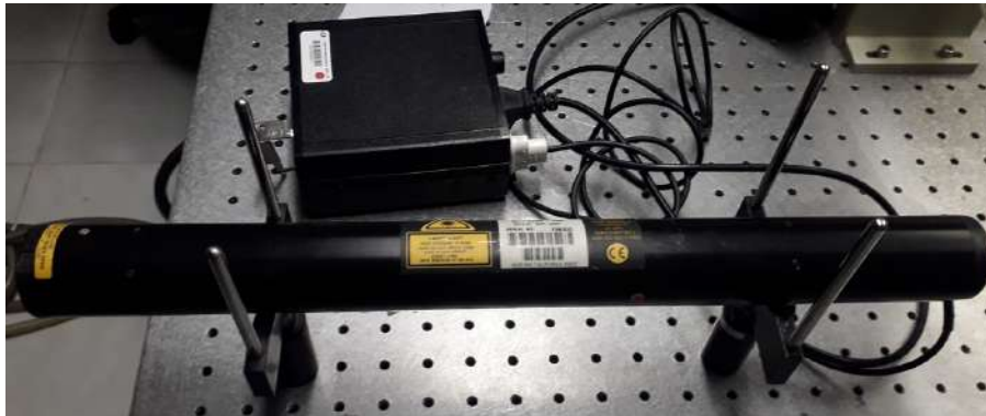
Figure 2.9: A 10 mW He-Ne Laser with a wavelength of 594 nm (Courtesy: CIO laser applications lab., Aguascalientes).
