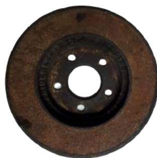
Figure 3.4: Corroded brake disk.
