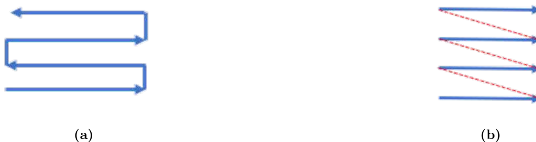
Figure 3.8: Laser scanning patterns used in the cleaning of carbon steel and cast iron (a) continuous, and (b) lineal.
