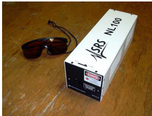
Figure 2.7: A nitrogen laser with a wavelength of 337 nm and 170 J pulse energy at 20 Hz (Image courtesy of [63]).
