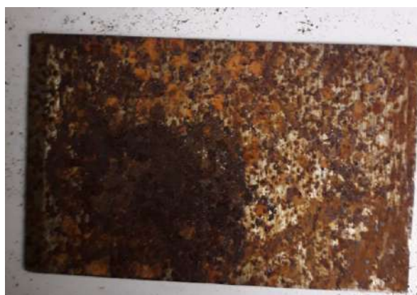
Figure 3.2: Corroded carbon steel plate.
