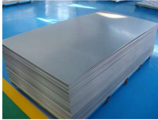
Figure 3.1: Uncorroded hot-rolled carbon steel plates (image courtesy of [110]).
