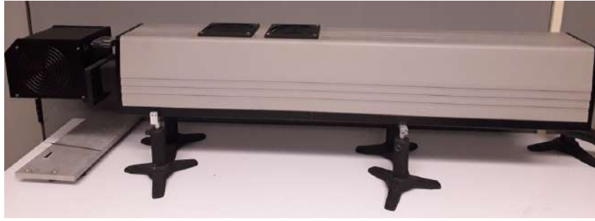
Figure 2.5: A 50 W pulsed CO_2 laser with a wavelength of 10.6 \mu m (Image courtesy of CIO laser applications lab., Aguascalientes).
