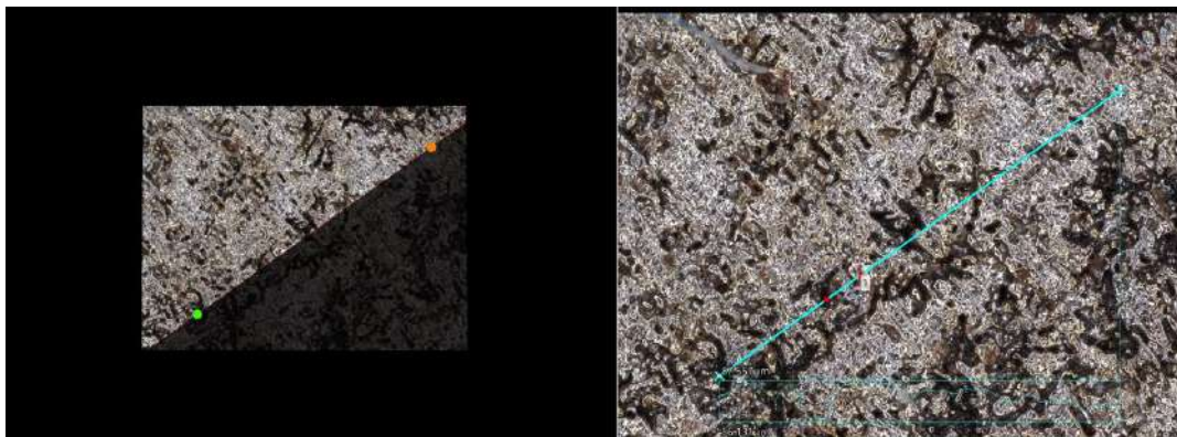
Figure 4.10: Optical analysis of the most cleaned grey cast iron sample R_{f3}
