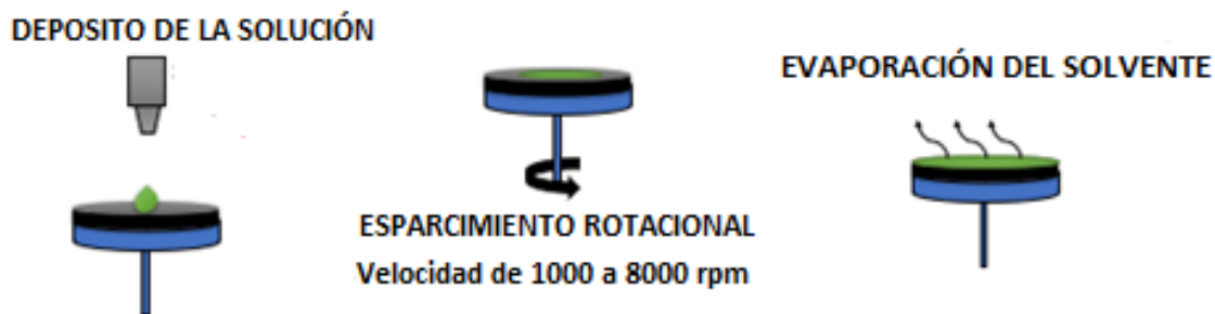
Figura 2.8: Diagrama de Spin Coating.
