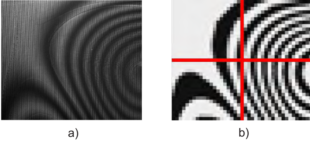
Fig. 5.21 a) Original shadow Moire fringe pattern, with resolution of 831 \times 971 pixels. b) Partitioned input fringe pattern, with a maximum number of fringe equal to 7.
