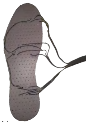
Figure 4.4. Wires resting on carved ducts on the insole.
