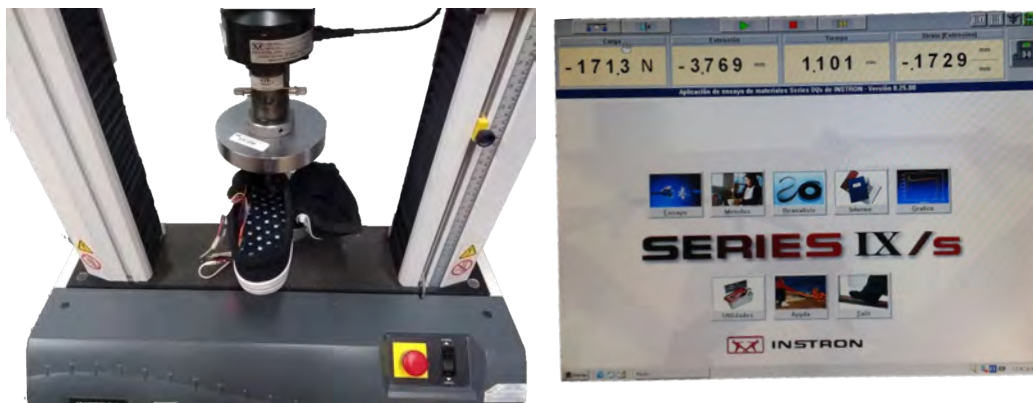
Figure 4.11. Footwear sensor characterization setup a) Half-opened footwear for in-shoe characterization on INSTRON 3369; b) INSTRON 3369 graphical interface.
