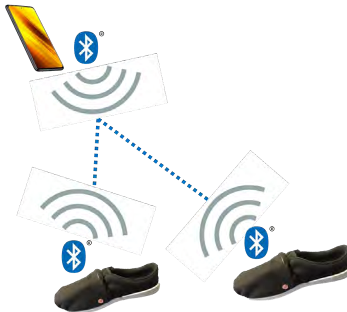
Figure 5.2. Point to Point network setup.
