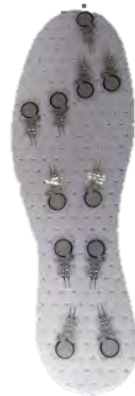
Figure 4.3. Sensors positioned on the cotton insole.
