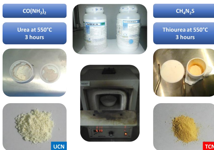
Figure 3.1 - Synthesis Process and g-C 3 N 4 Products
