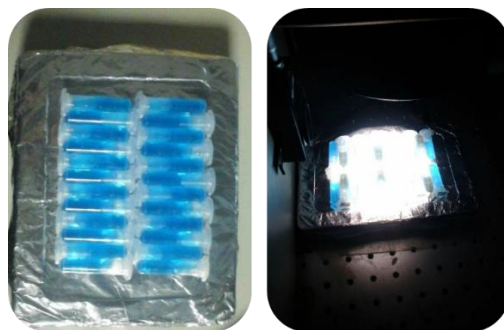
Figure 3.5 - Eppendorf tubes subjected under the solar simulator
