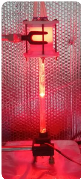
Figure 6.1 - A waveguide photocatalysis reactor
