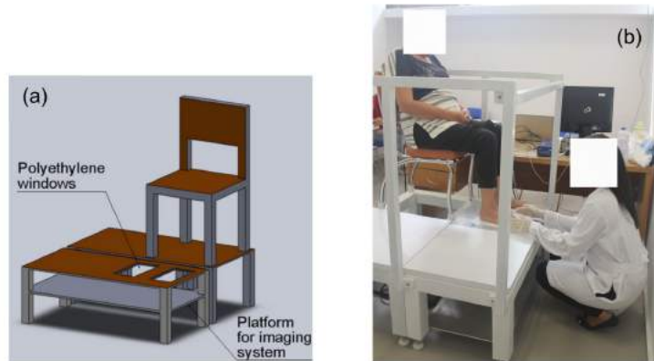
Figure 4.1: MMAT scanner v1. (a) Platform setup design considering a chair, two polyethylene windows and a platform for the imaging system. (b) Terahertz images acquisition during the MMAT technique proof-of-concept study.
