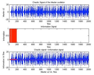
**Fig. (5).** Chaotic signal of the master oscillator, signal to transmit, and the transmitted signal with information.
