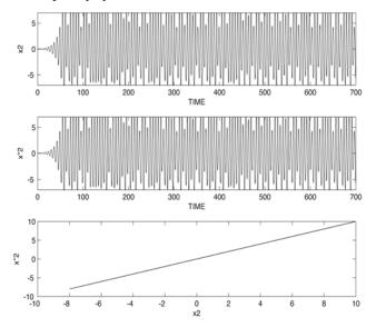
Fig. (2). Chaotic time series of master and slave variables and  $x_2$  versus  $x_2$  demonstrated complete synchronization.
