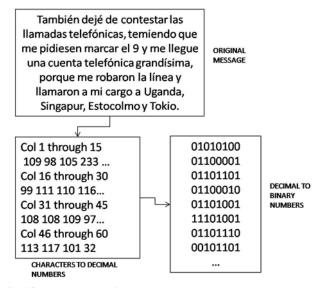
Fig. (4). The message first is encoded to the decimal numbers and then to the binary numbers.
